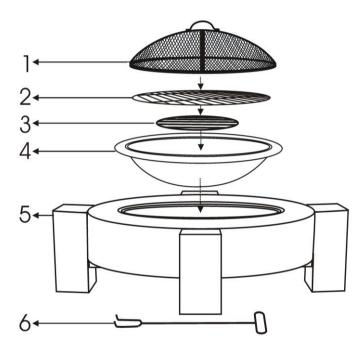
**STEP 1-** Place the MGO stand (5) on a permanent flat, level, heat resistant, non flammable surface away from flammable items.
