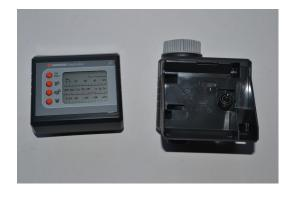
New style, remove front then release case by carefully releasing 4 plastic catches
