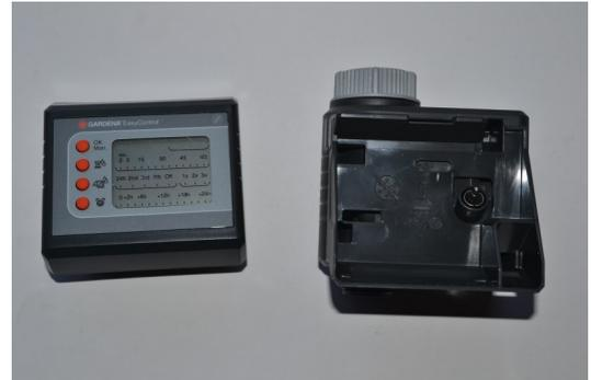
New style , remove front then release case by carefully releasing 4 plastic catches
